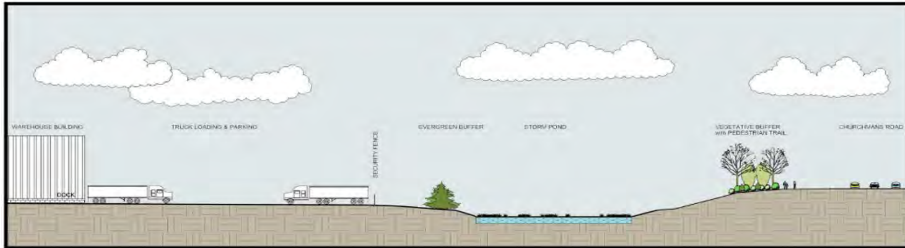
A SECTION / ELEVATION A LOADING AREA with EVERGREEN BUFFER, STORMWATER POND and VEGETATIVE BUFFER with PEDESTRIAN TRAIL SCALE
